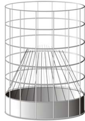
Figure 4: Entrance valve to roost capsule for Myna Trap (Scale: mesh = 25 mm)
